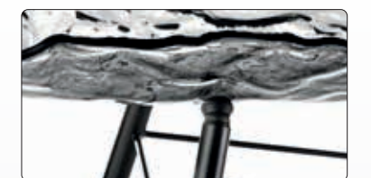
Hinged beams at the upper side of the trestle can be adjusted individually to the shape of bowls and platters
